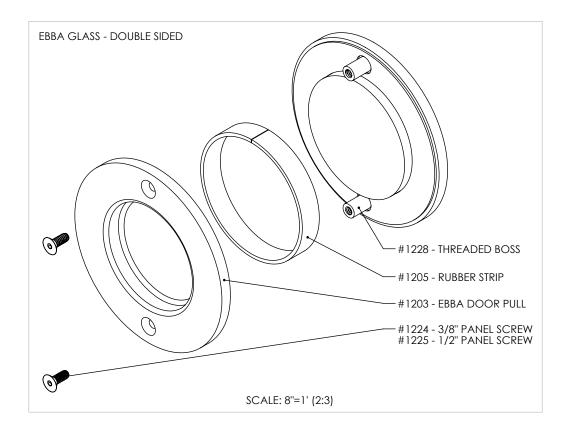
GLASS PANELS MUST BE FLAT POLISHED AND HAVE A 1MM CHAMFER ON ALL EDGES.
