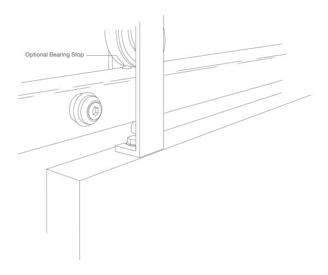
1 Install Optional Bearing Stop on top edge of track to stop your panel in any desired location.
