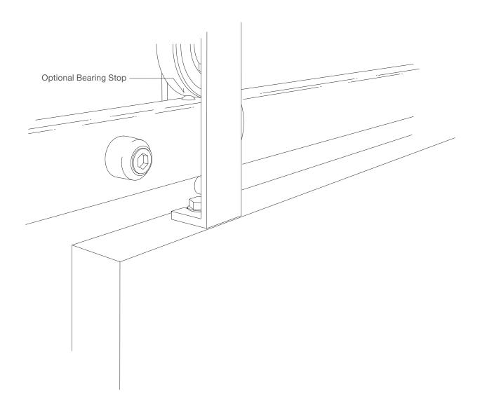
1 Install Optional Bearing Stop on top edge of track to stop your panel in any desired location.
