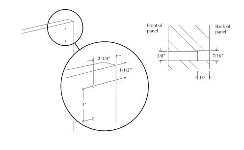
Install safety stop to top of door panel. Do not over-tighten screw.
