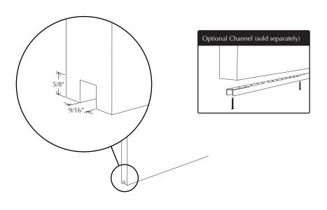
Drill holes in door panel for mounting trolleys.
