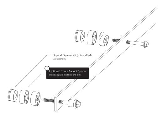
Black bumpers included in Trolley Stop Track Mount Kits are designed to stop the door panel. Position them at end of track, or where you want door panel to stop.
