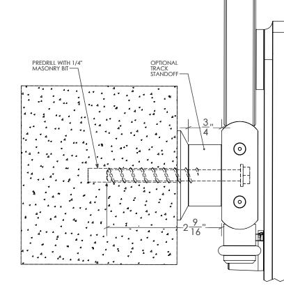
**Concrete Wall** Concrete and masonry walls must be solid and thicker than the minimum required thread engagement of 1-1/2".Concrete kits include 5/16" x 3" screw-in anchors.
