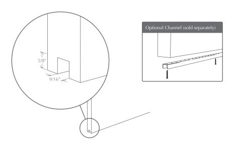
7 Drill holes in door panel for mounting trolleys.
