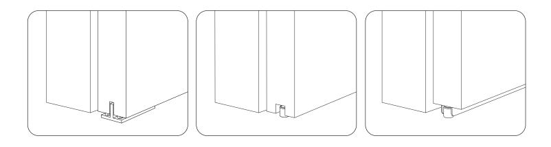
Installation of a door guide is required, and must always be engaged for safety.
