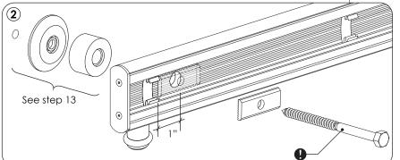
Krownlab offers a range of mounting point fasteners for different wall conditions. Lag screws for walls with wood blocking are illustrated here.
