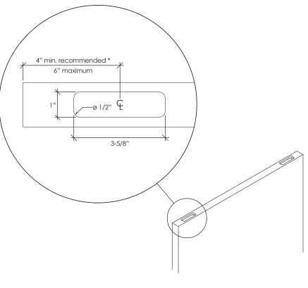
\* Facilitates easier door guide post installation in step 20.
