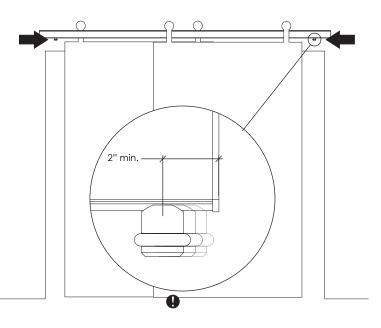
Not tightening door stops to provided specs can cause the door to slide off the end of the track and cause damage and a safety hazard.
