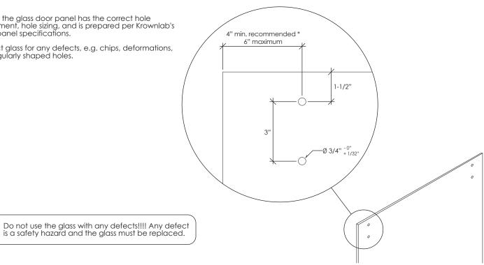
\* Facilitates easier door guide installation in step 19.
