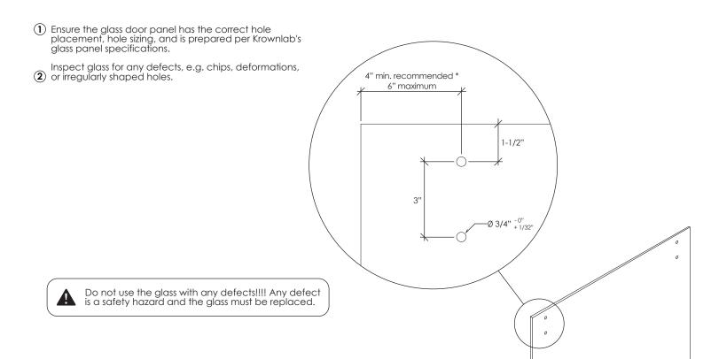
\* Facilitates easier door guide installation in step 21.
