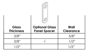
Optional glass panel spacer is solely intended for 3/8" thick door panels.
