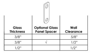
Optional glass panel spacer is solely intended for 3/8" thick door panels.
