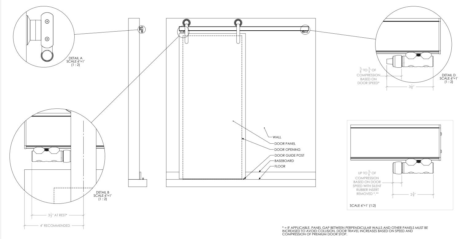
\*\* = REMOVING SILENT RUBBER INSERT WILL REMOVE THE SILENT FEATURE, BUT MAY BE A NECESSARY ADJUSTMENT TO REDUCE POSSIBLE EXTRA DOOR TRAVEL. THE ENERGY ABSORBING FEATURE OF THE PREMIUM DOOR STOP WILL REMAIN IN THIS CONFIGURATION.
