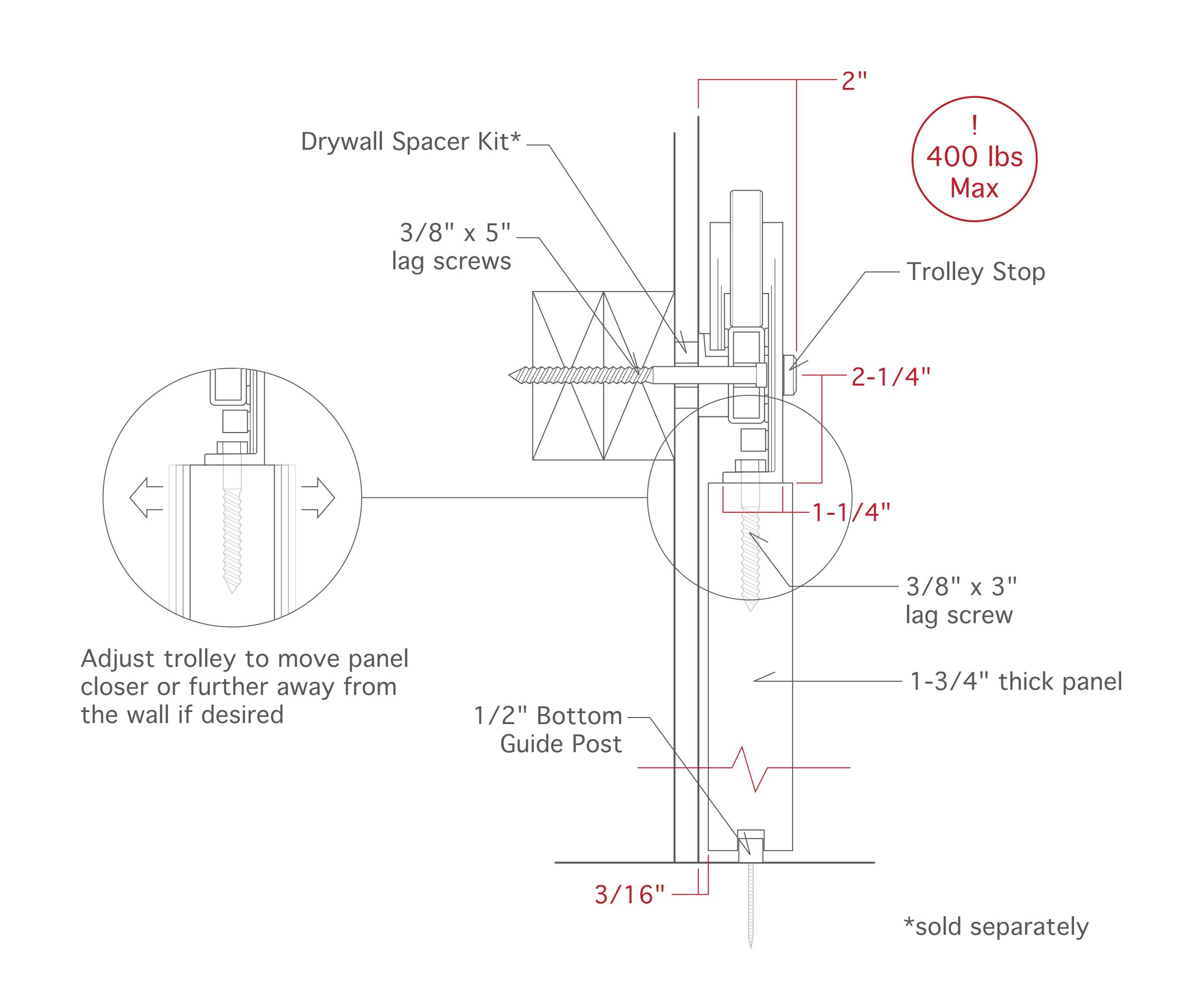
Section AA with single Track Mount Spacer Maximum panel weight is 400 lbs
