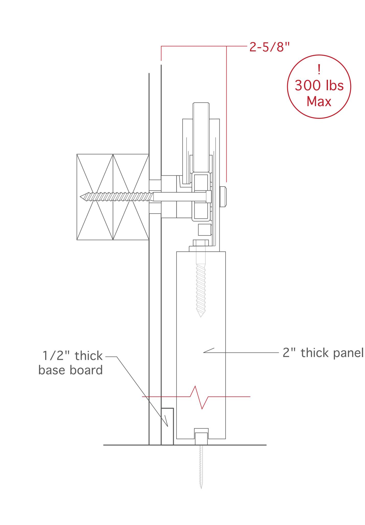
Section AA with double Track Mount Spacer
