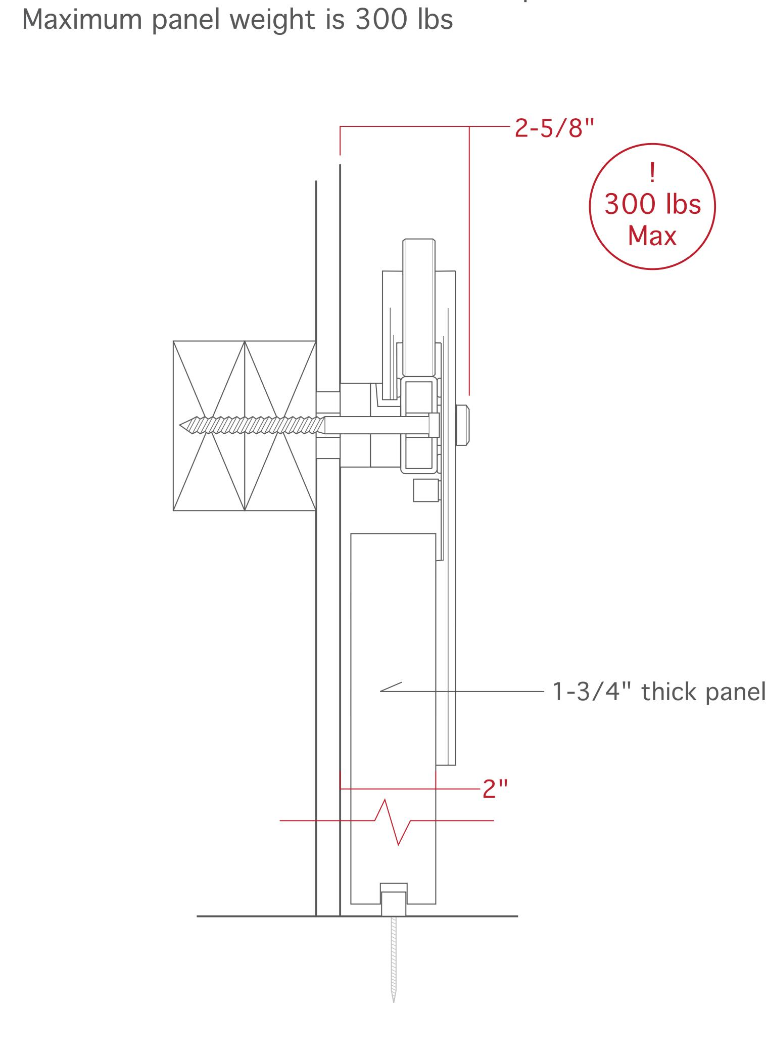
Section AA with double Track Mount Spacer
