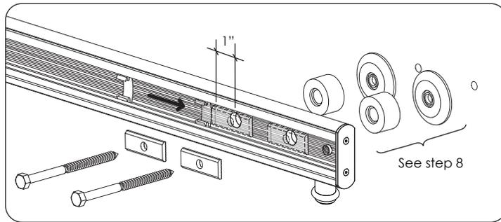
**⚠** Krownlab offers a range of mounting point fasteners for different wall conditions. Lag screws for walls with wood blocking are illustrated here. Contractor or other qualified professional to ensure suitability of provided fasteners for site-specific wall conditions.
