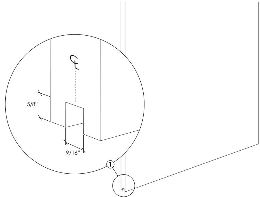
**⚠** Installation of a floor guide is mandatory. Door panel has to be engaged by the floor guide along its entire travel. Not following the above instructions can cause a hazardous condition.
