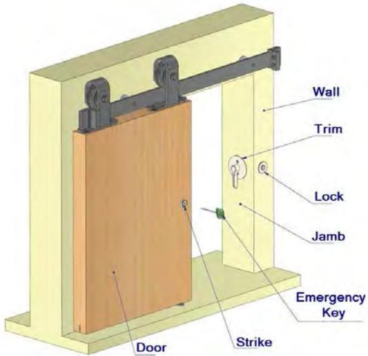
Installation based on barn door application where doors are hung on the **OUTSIDE** of the room.
