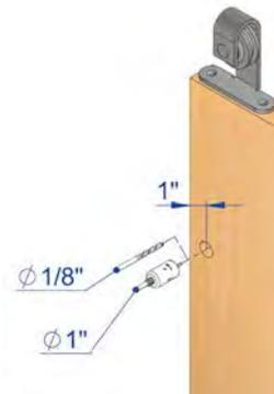
6.3) With the pilot hole as a guide, use a 1/4" bit to drill a hole from the outside to connect with the strike bore hole.
