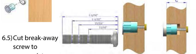
6.5) Cut break-away screw to appropriate door thickness. DO NOT OVER TIGHTEN
